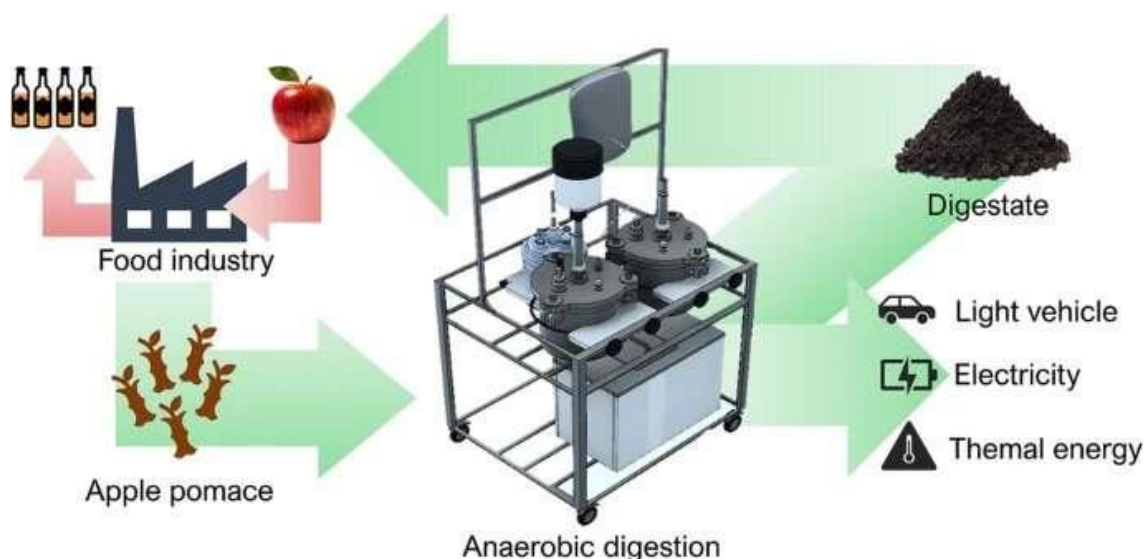
Figure 51: Process for valorisation of apple pomace for bioenergy
